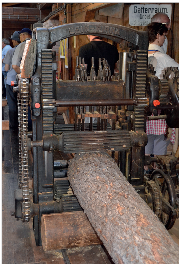
Fig. 3. The vertical gang saw, in a very crowded saw mill! (G. Hackney).
