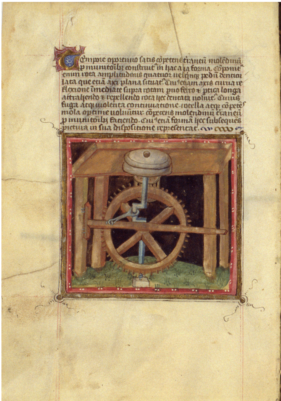
Fig. 3. ms. Vat. Lat. 5961 fol. 40v: Hand mill with crank and connecting rod for grinding in fortresses.
