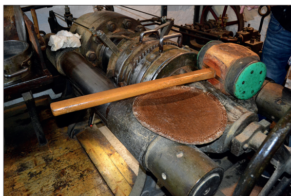
Fig. 5. The horizontal press with pans in place; the huge hammer is used to knock the pan lids on tight (G. Hackney).
