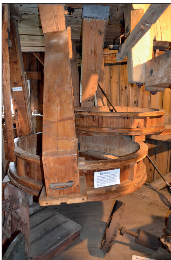
Fig. 18. The pair of hopper boys in Kottmarsdorf windmill (G. Hackney).
