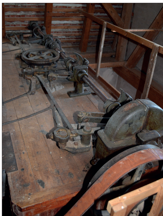
Fig. 7. The complicated system of gears, levers and cams which operate the dust extractor socks from above (G. Hackney)..
