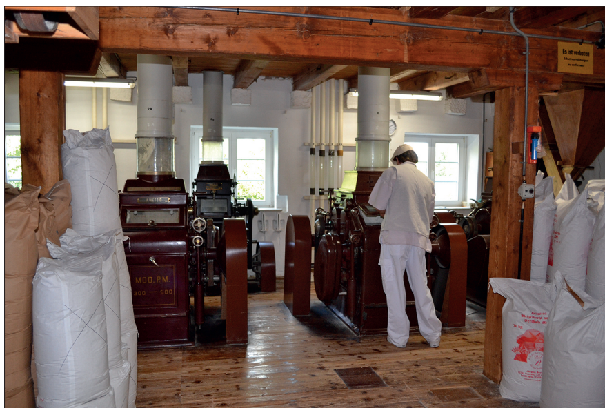
Fig. 9. Berthold-Mühle; Jurgen operating roller mills (G. Hackney).
